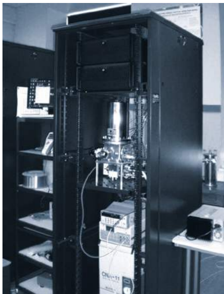
ITMO experimental quantum cryptography set with SSPD detector.
